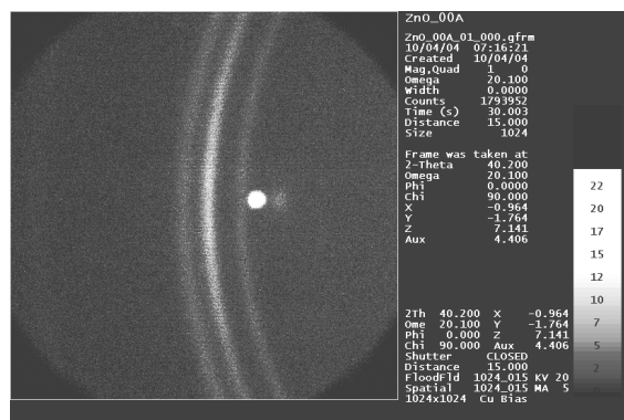
Fig 5. Sputtered ZnO thin films showed columnar polycrystalline structure with preferred orientation in \langle 002 \rangle direction
